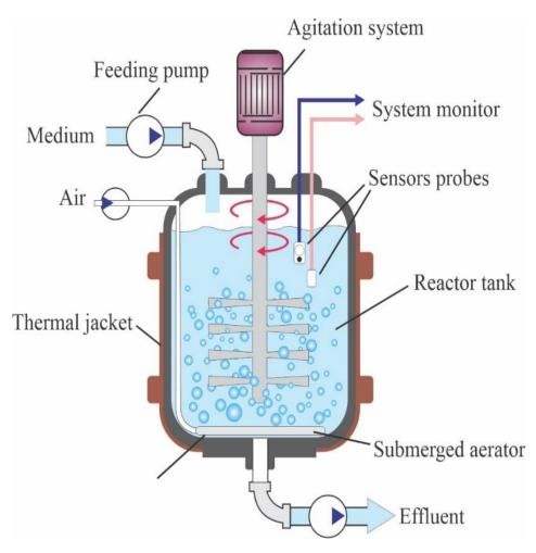
Figure 9. Continuous stirred tank bioreactor (Adapted from Saran et al.) [98]
