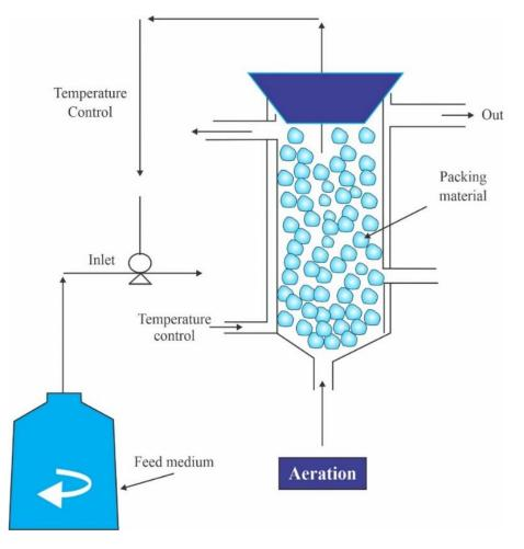
Figure 5. Packed bed fermenter (Adapted from Siegel and Robinson) [92]
