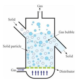
Figure 4. Fluidized-bed fermenter (Adapted from Kowng) [94]
