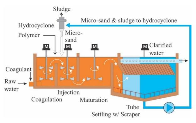
Figure 8. Ballasted floc bioreactor (Redrawn from Krüger published in Capodaglio) [97]
