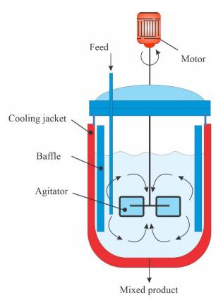
Figure 1. Continuous stirred tank fermenter (Adapted from Tavoosi et al.) [91] Gas flow outlet
