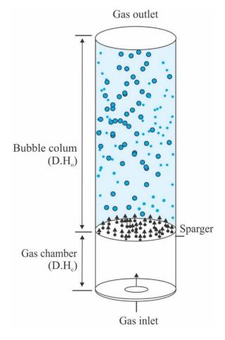
Figure 3. Bubble column fermenter (Adapted from Wilkinson et al.) [93]
