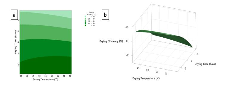
Figure 1. Tapioca cracker drying energy efficiency: (A) Two-dimensional plots and (B) three-dimensional plots
