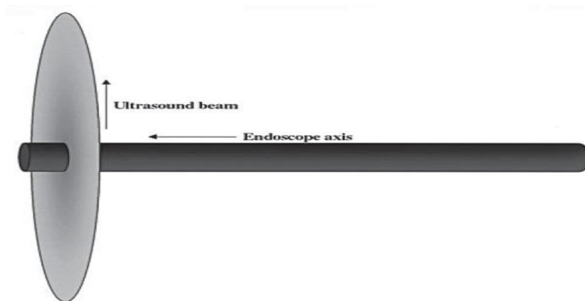
Figure 2: The radial echoendoscope scans at an axis perpendicular to the endoscope shaft.
