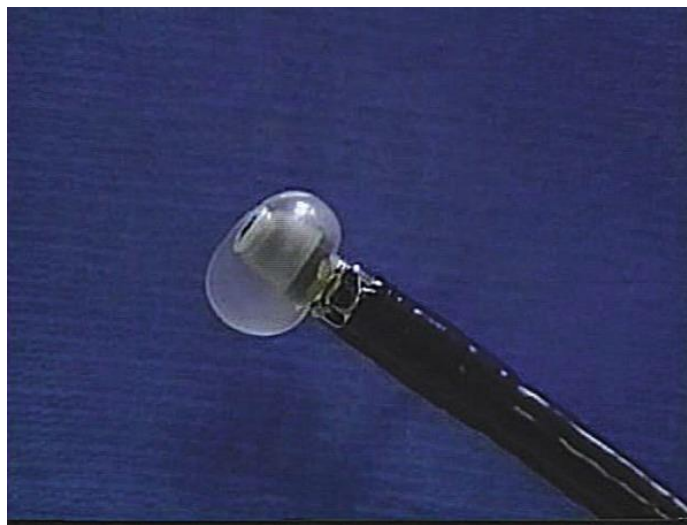
Figure 1: The electronic radial echoendoscope (Olympus Corporation, Tokyo, Japan).
