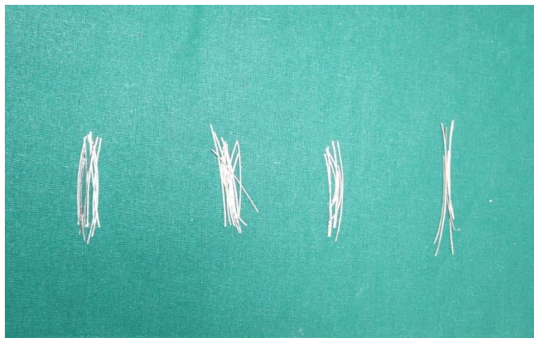
Fig 4: Retrieved archwires were cut into segment of 40mm each after intraoral engagement in orthodontic brackets for six weeks.
