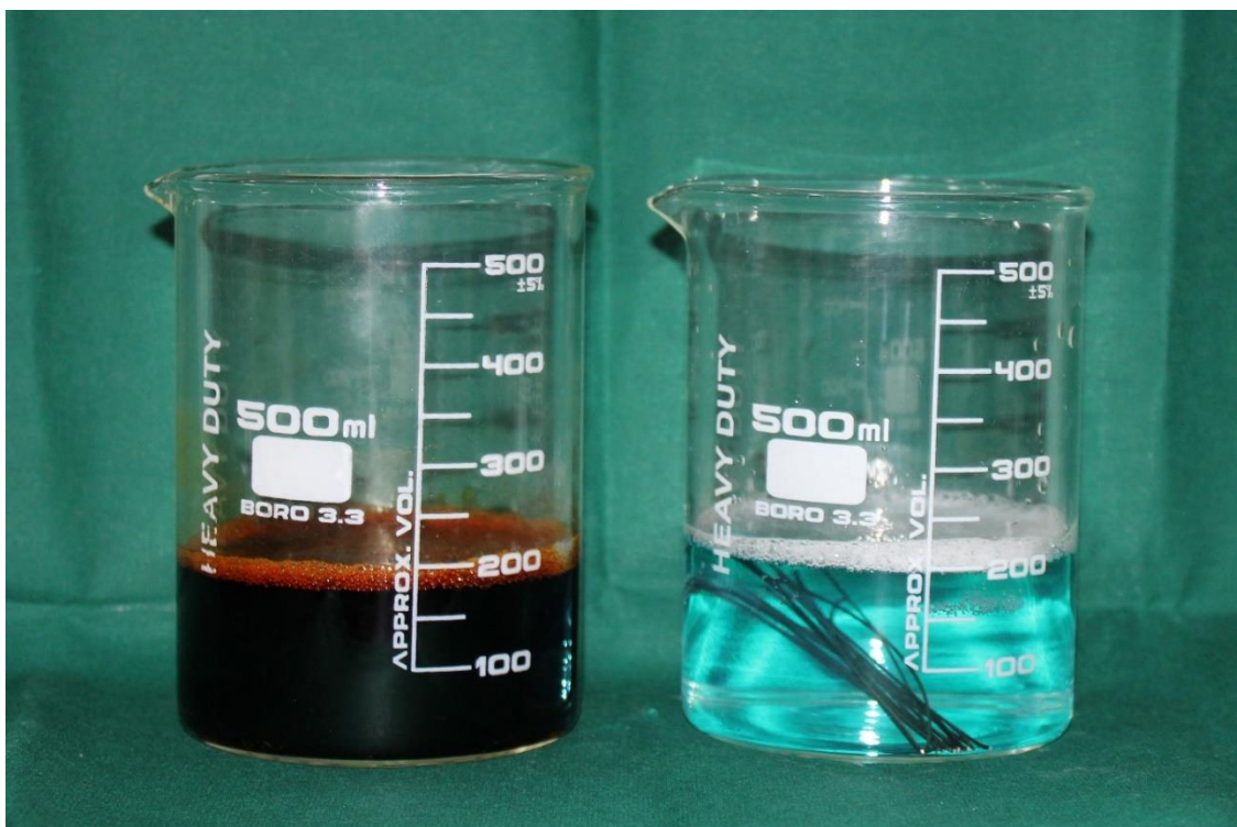
Figure 2. The test groups immersed in the mouthwashes (povidone-iodine and chlorhexidine) for one and half hour
