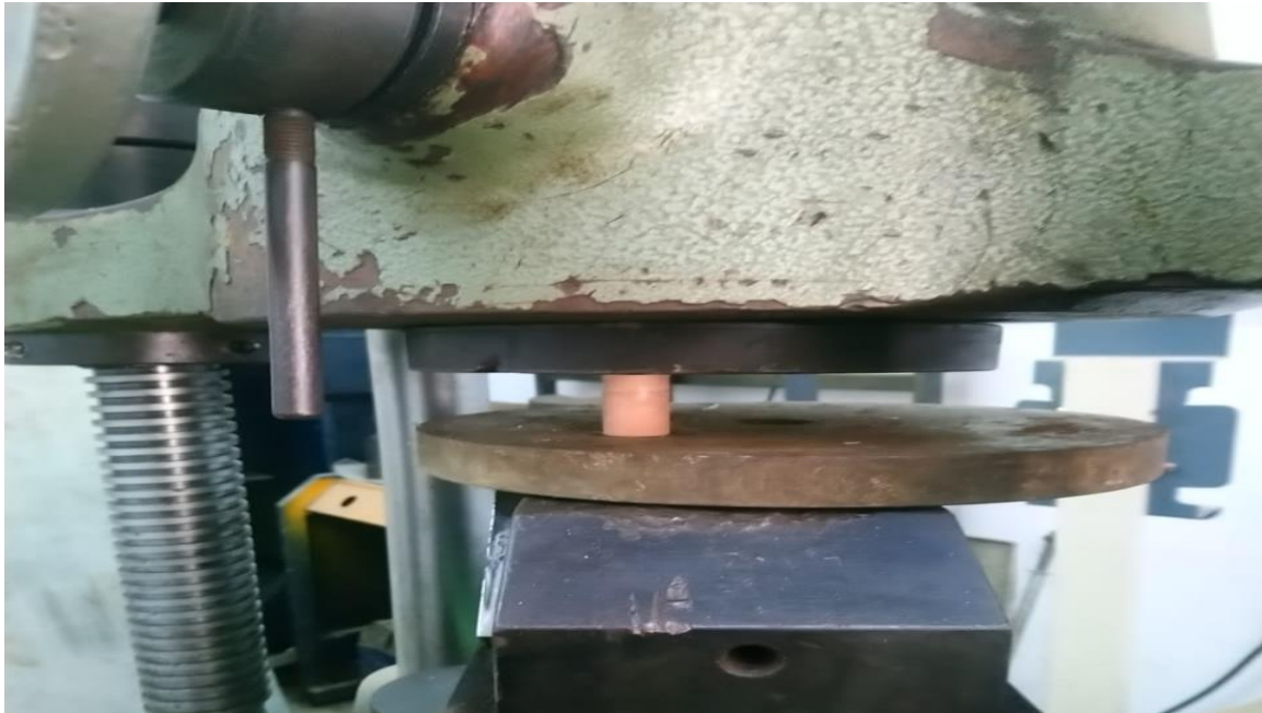
Figure 3: A compressive strength test of reinforced sample
