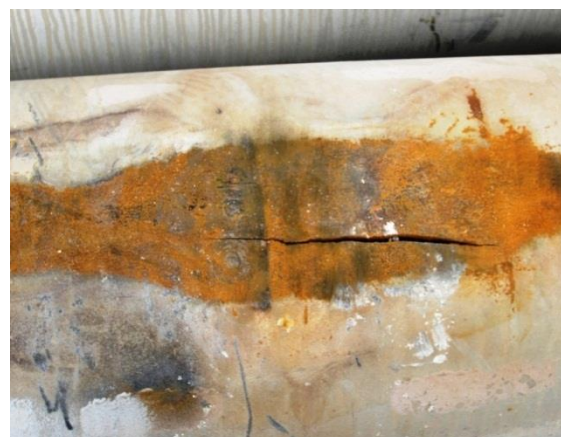
Figure1. Damaged support (left) and rupture on pipeline at 6 o' clock position (right)
