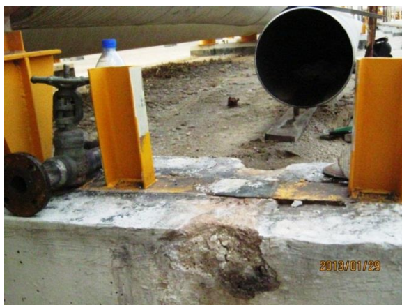
Figure1. Damaged support (left) and rupture on pipeline at 6 o' clock position (right)
