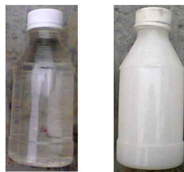
Fig. 1(a): uncoated container, Fig. 1(b): TiO 2 -coated container
